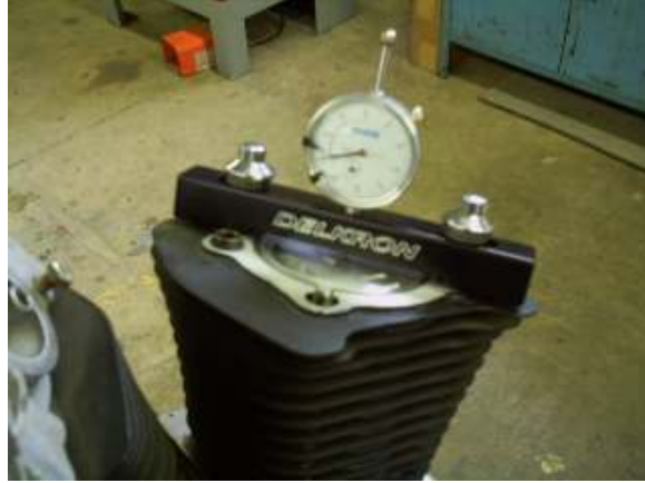
LOCATING TRUE “TDC” WITH HEADS REMOVED
