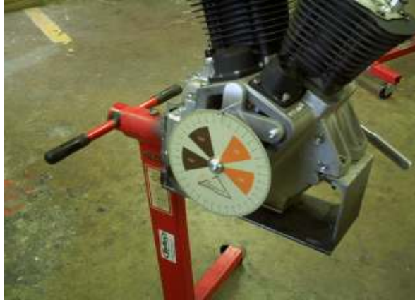
SETTING BREATHER GEAR TIMING
